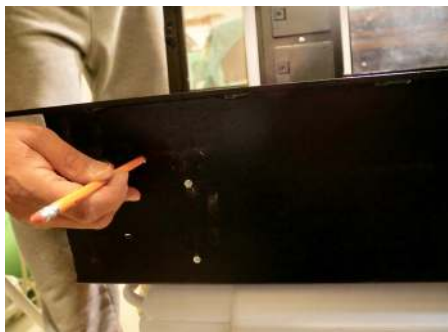
With a sharp object, pierce the material on the other side of the four holes on each side, top and bottom.
