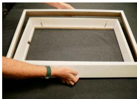
Separating outer, sloped part of Frame from inner Frame box.
