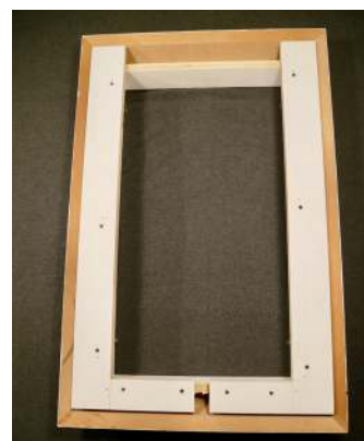
Back of assembled frame. Note hole at bottom for wire.
